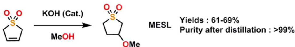
Scheme 1. Synthetic pathway used for MESL.
