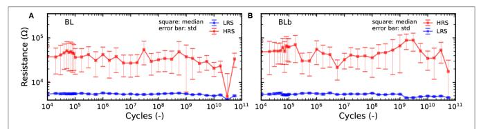
**FIGURE 7 | (A,B)** Mean resistance value of the BL and BLb device over 10 thousand cycles for measurements of a device pair over  $5 \times 10^{10}$  cycles. RESET voltage of 1.5V, SET current of  $200 \,\mu A$ , and programming time of  $1 \,\mu s$ .
