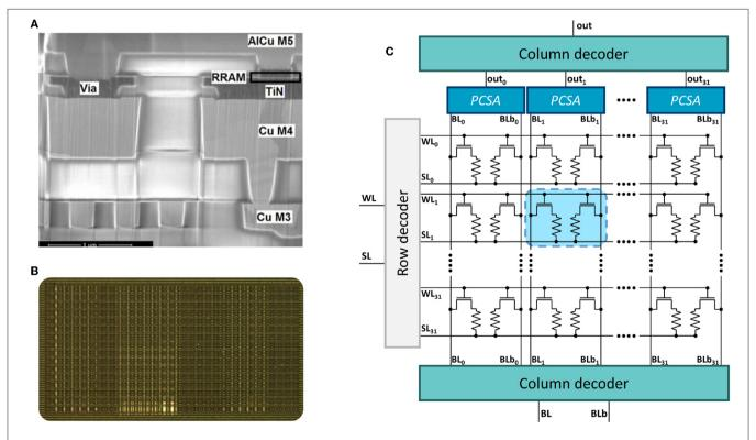
FIGURE 1 | (A) Scanning Electron Microscopy image of the back-end-of-line of the CMOS process integrating an OxRAM device. (B) Photograph and (C) simplified schematic of the one kilobit in-memory computing-targeted memory array characterized in this work.
