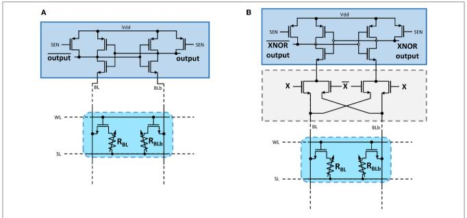
FIGURE 2 | (A) Schematic of the precharge sense amplifier used in this work to read 2T2R memory cells. (B) Schematic of the precharge sense amplifier augmented with an XNOR logic operation.
