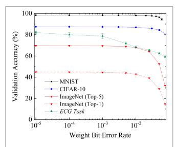
**FIGURE 9** | Recognition rate on the validation datasets of the fully connected neural network for MNIST, the convolutional neural network for CIFAR10, and AlexNet for ImageNet (Top 5 and Top 1) and in the ECG analysis task, as a function of the bit error rate over the weights during inference. Each experiment was repeated five times; the mean recognition rate is presented. Error bars represent one standard deviation.
