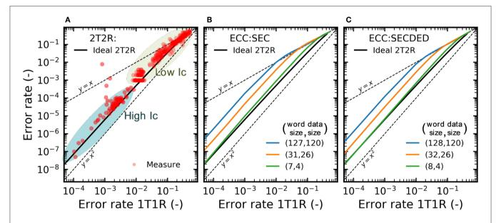
FIGURE 8 | (A) Experimental bit error rate of the 2T2R array, as measured by precharge sense amplifier, as a function of the bit error rate obtained with individual (1T1R) RRAM devices under the same programming conditions. The detailed methodology for obtaining this graph is presented in the body text. Bit error rate obtained with (B) Single Error Correcting (SEC) and (C) Single Error Correcting Double Error Detection (SECDED) ECC as a function of the error rate of the individual devices.
