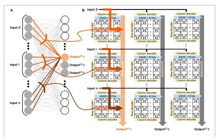
**FIGURE 3 (A)** Schematization of the implemented Binarized Neural Network highlighting connections to one specific neuron. **(B)** Schematization of the full architecture to implement the Binarized Neural Network in the "parallel to sequential" configuration. The system assembles a memory block surrounded by logic circuits and moves minimal data between the blocks. The architecture is presented with three rows and three columns (i.e., N = M = 3) of kilobit memory blocks (i.e., n = 32).
