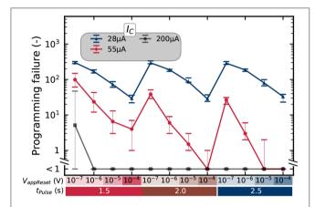
FIGURE 5 | Number of errors for different programming conditions, as measured by precharge sense amplifier, for a 2T2R configuration on a kilobit memory array. The "< 1" label means that no errors were detected. The error bars present the minimum and maximum number of detected errors over five receitions of the experiments.
