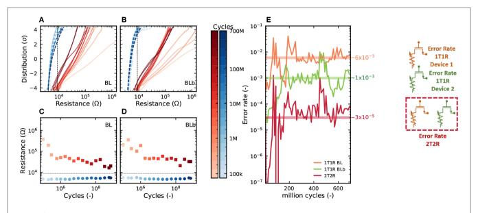
**FIGURE 6 | (A,B)** Distribution of resistance values, **(C,D)** mean resistance value, and **(E)** mean bit error rate over 10 million cycles, as measured by precharge sense amplifier, in the 2T2R configuration, as a function of the number of cycles for which a device has been programmed. RESET voltage of 2.5 V, SET current of 200  $\mu$ A, and programming time of 1  $\mu$ s.
