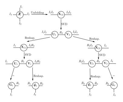
Fig. 5. TT-HSVD applied to a 4-order tensor.
