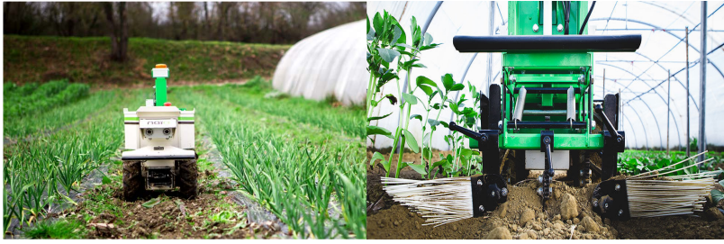
Fig. 1 Oz in operation. Left: front view; right: back view with tools.
