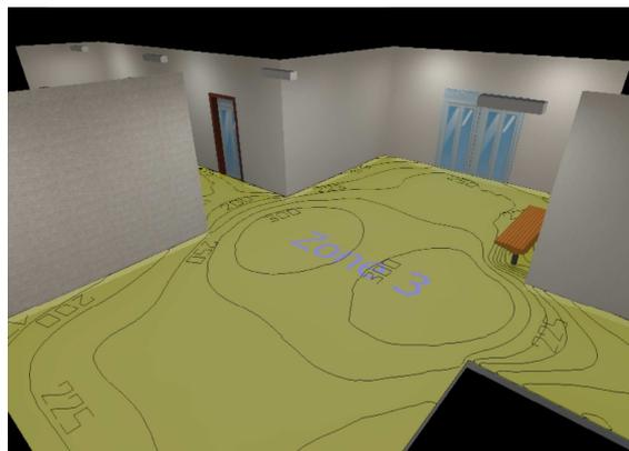
Fig. 1. The classical design for interior lighting system, with vertical illuminance in lux for the working plane.
