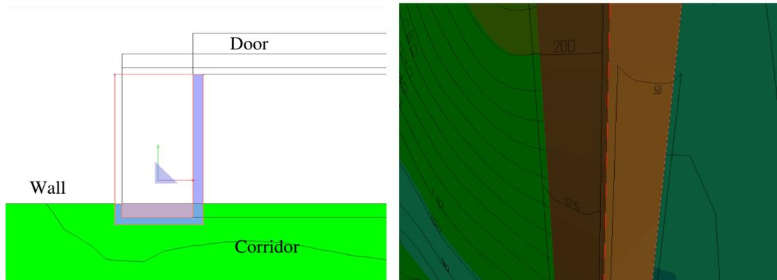
Fig. 4. Building the frame of the door (with “extrusion object”) on the left, and illuminance in lux on the calculation object (right).
