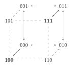
We can now observe that IC is not geodetic: the shortest paths between (100) and (111) in  $\mathcal{G}_{\mathcal{D}}^1$  pass through either (110) or (101), which however are not nodes of  $\mathcal{G}_{IC}^1$ .
