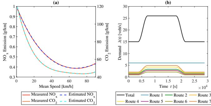
Fig. 2. Emission factors curves of NO<sub>x</sub> and CO<sub>2</sub> (left column) and demand profiles used in the case study (right column).
