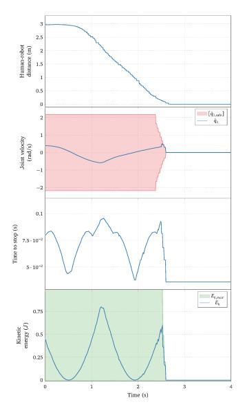
Fig. 5. Human-robot separation distance, joint velocity constraints of joint 1, robot maximum stopping time, and robot kinetic energy versus time. The red area represents the safe velocity for joint 1 computed from eq. (5). The green area represents the maximum kinetic energy that the robot can acquire according to the joint velocity limits.
