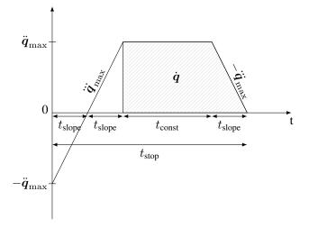
Fig. 2. Worst case  $(\dot{q} = -\dot{q}_{\max}, \ddot{q} = -\ddot{q}_{\max})$  maximum deceleration profile until reaching a complete stop.
