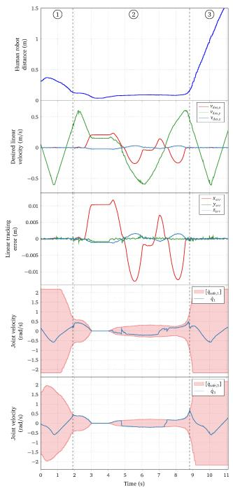
Fig. 6. Human-robot separation distance, desired operational velocity ( $v_{des}$ ), trajectory tracking error and joint velocity constraints of joints 1 and 3 versus time. The red area represents the safe velocities for the joints.
