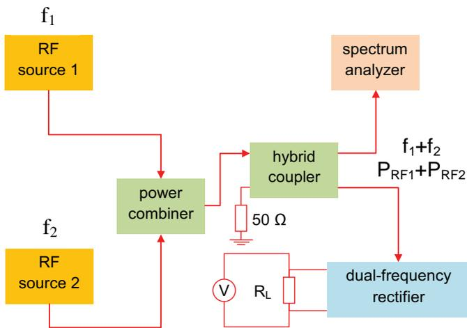
Figure 4. Measurement setup
