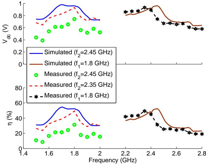
Figure 7. Simulated and measured output dc voltage and efficiency against frequency
