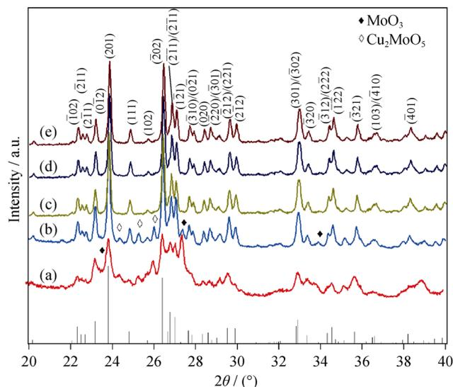
**Fig. 3.** XRD patterns of  $\text{CuMoO}_4$  powders heat-treated at (a) 300, (b) 420, (c) 450, (d) 500, and (e) 550°C for 6 h. The standard pattern for  $\text{CuMoO}_4$  (JCPDS file No. 73-0488) is provided at the bottom of this figure.
