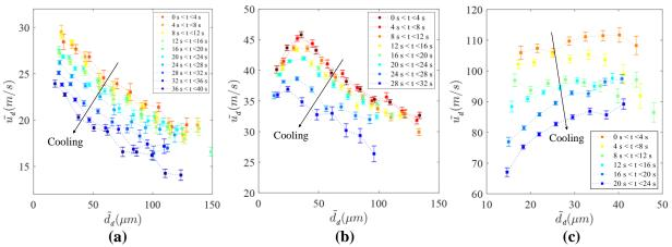
Figure 5. Correlation of droplets diameter and velocity downstream of Part II during the cooling phase for each configuration: (a) 0%, (b) 61% and (c) 90% blockage
