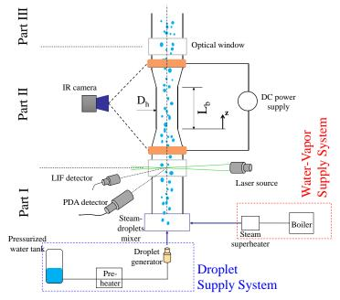
Figure 2. Schematic drawing of the COLIBRI experimental apparatus.
