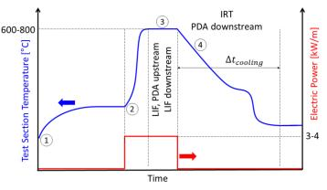
Figure 3. Test procedure. (1) Start of the steam flow; (2) Start of the droplets injection and heating of the test section; (3) Measurement of the droplets characteristics; and (4) Cooling experiment.
