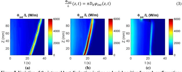
Figure 7. Variation of the internal heat dissipation in time and axial position for each configuration: (a) 0%, (b) 61% and (c) 90% blockage ratio (dotted black line: rewetting front).
