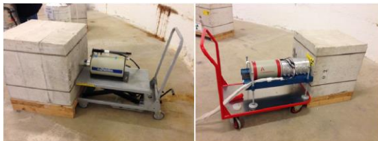
Fig. 2. Coaxial HPGe detector (left) and planar (right) measurement setup in Bessines' calibration station. The coaxial detector head is inserted inside the block hole (see Fig.5) while the planar detector is outside, in contact with the concrete block (Fig.6)
