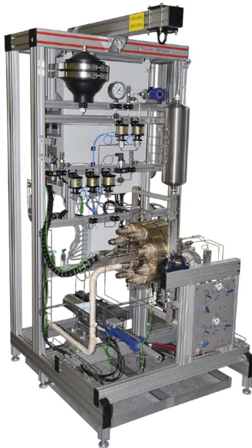
Figure 9: View of the fatigue new bending device FABIME2E
