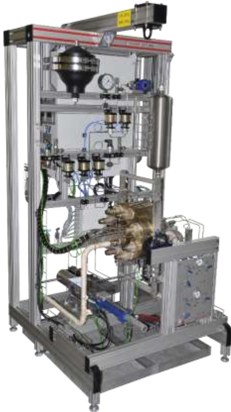
Figure 7. View of the fatigue new bending device FABIME2E
