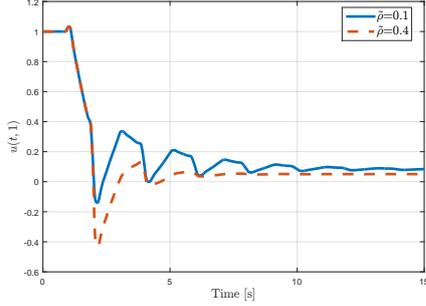
Fig. 6. Evolution of the output  $u(t,1)$  in the absence of noise with a disturbance  $d_3 = 0.1$  for different values of  $\tilde{\rho}$  with  $k_I = 0$  and  $\epsilon = 1$ .
