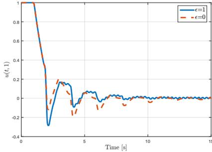
Fig. 7. Evolution of the output  $u(t,1)$  in the absence of disturbance along with a high frequency noise for different values of  $\epsilon$  with  $k_I = 0$  and  $\tilde{\rho} = 0.2$ .
