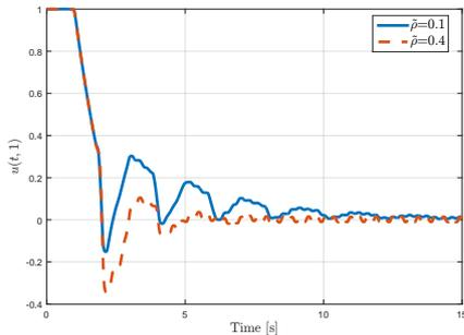
Fig. 8. Evolution of the output  $u(t,1)$  in the absence of disturbance along with a high frequency noise for different values of  $\tilde{\rho}$  with  $k_I = 0$  and  $\epsilon = 1$ .
