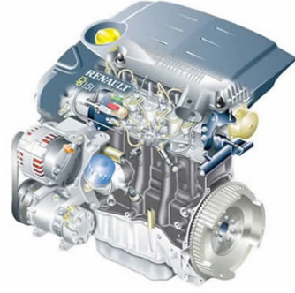
Figure 2: Reference engine (belt, accessories and bracket are in the lower left-hand corner)
