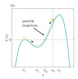
Fig. 2 (a) Potential  $U(\phi)$  with a false vacuum state  $\phi_1$  and a true vacuum state  $\phi_3$ . Vacuum decay corresponds to instantons solutions to Eq. 3 interpolating  $\phi_1$  and  $\phi_3$ . (b) A fictitious particle moving in the potential  $V(\phi) = -U(\phi)$ . For the instanton to exist, the particle should pass the bottom of the valley  $V(\phi_2)$  and come to rest at time infinity on top of the maximum  $V(\phi_1) = 0$ .
