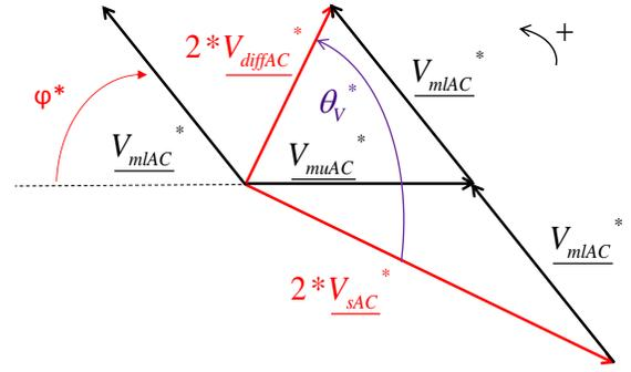
Fig. 8. Phasor diagram of the AC M2DC voltages.
