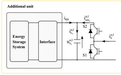
Fig. 2. Structure of an Energy Storage Submodule (ES-SM)
