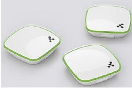
Fig. 1. BLE beacons by Kontakt.io used for data collection.
