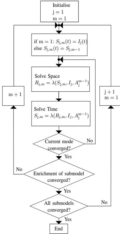
Fig. 1. Alternating scheme to determine linear PGD representation.
