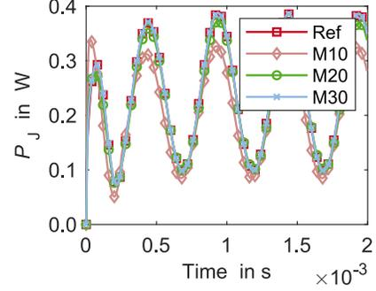
Fig. 3. Eddy current losses in the conductive sample.
