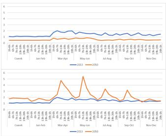
Fig 2 Synchronism indicator in 2013 (blue) and 2050 (red) for BAU (top) and 100% REN (bottom) scenarios. The assesment is plotted for relevant time slices of the year, including a "critical week" with low solar and wind production and no imports.
