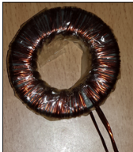
Fig. 9. Realized coil of 2.48 mH.
