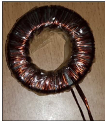
Fig. 9. Realized coil of 2.48 mH.
