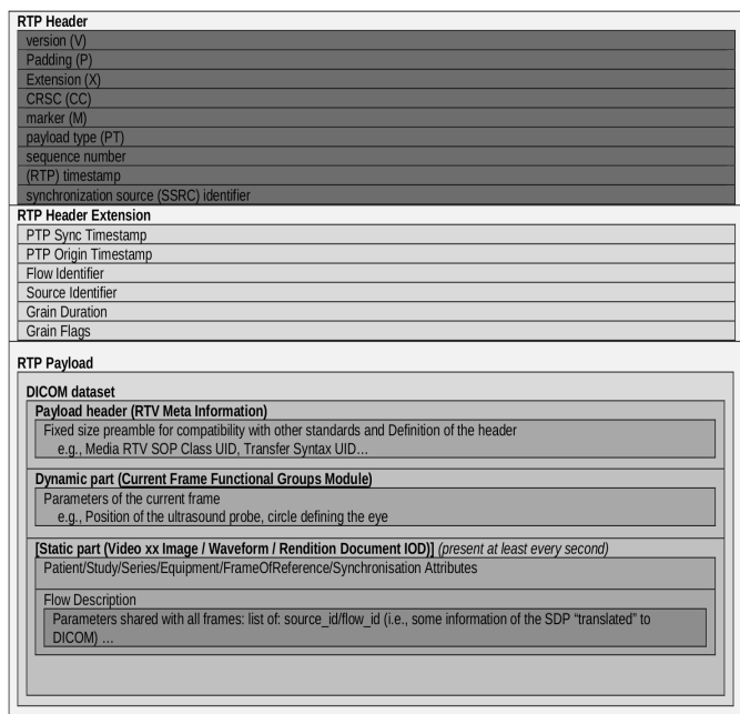
Fig. 5. DICOM dataset encapsulation within RTP
