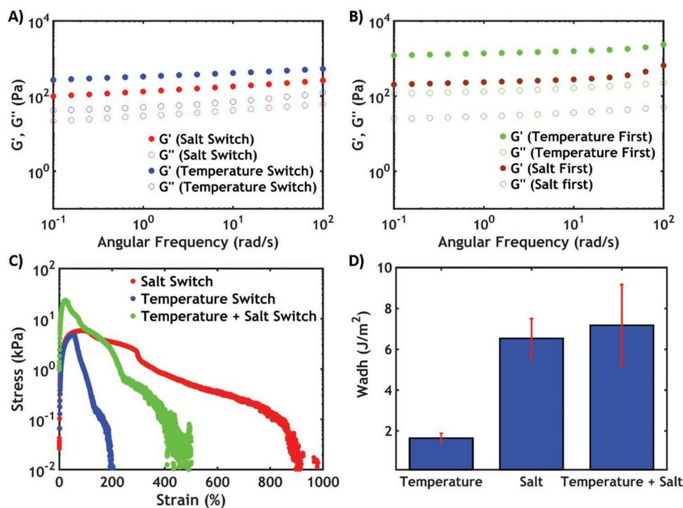
**Figure 3.** Mechanical and adhesive behavior of the graft copolymer complex coacervate phase in response to different triggers. A) Frequency sweeps obtained after either a temperature or a salt switch. B) Effect of the history of the setting process on the rheological properties when applying a combined temperature and salt trigger. C) Adhesion performance and D) work of adhesion measured after different environmentally triggered setting processes.
