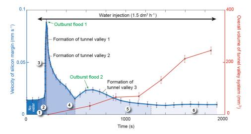
**Figure 5.** Progressive expansion of overall volume of tunnel valley system vs. velocity of silicon margin through the experiment. The circled numbers correspond to the six stages of the proposed ice stream life cycle.
