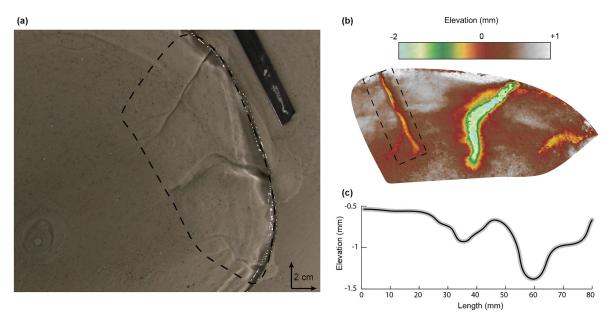
**Figure 4.** Digital elevation model (DEM) of an experimental tunnel valley and its associated longitudinal profile. (a) Snapshot of the tunnel valley system. (b) DEM of the tunnel valley corresponding to the one highlighted by a dashed box in (a). (c) Undulating longitudinal profile of the tunnel valley bottom extracted from the DEM in the dashed box shown in (b).
