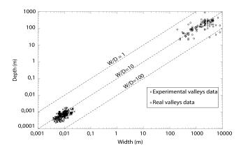
**Figure 10.** Width-depth ratios for experimental and natural tunnel valleys. References for the natural valleys are given in the supporting information.
