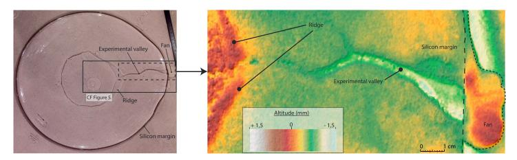
Figure 3. Surface photograph of an experiment and DEM of an experimental valley produced by stereo-photogrammetry.
