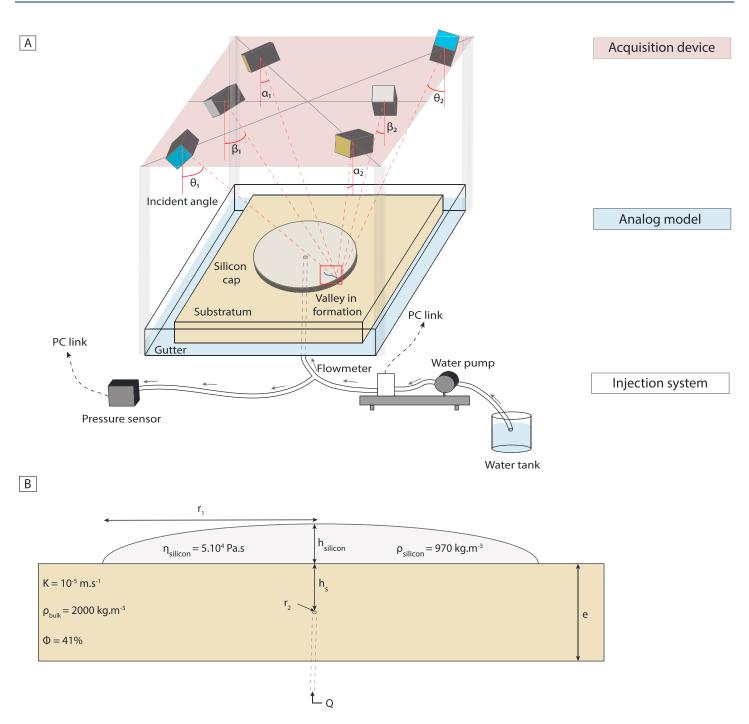
**Figure 1.** Experimental apparatus. (a) Acquisition device, analog model, and water injection system. Grey arrows symbolize the water flow direction. The photographic device is composed of three pairs of cameras focused on the valleys in formation. The incident angle is measured for every camera and used for the correction of the digital elevation model. (b) Transverse section of the analog model and associated variable and parameters.
