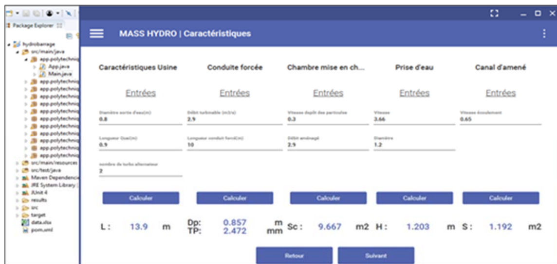
Figure 13: Module of design of Weir, intake, channel, fore bay, penstock and power house (software available in French version only).
