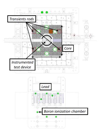
Fig. 1. Experimental boron ionization chambers near CABRI core
