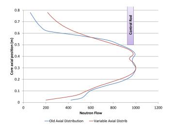
Fig. 9. Calculated axial distribution compared to the old axial distribution
