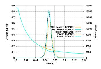
Fig. 12. Effect of the TOP effect model on the power transient calculation
