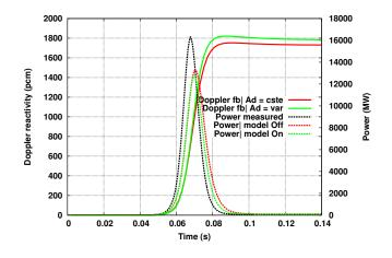
Fig. 8. Effect of Doppler model on the power transient calculation
