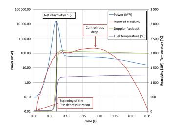
Fig. 3. Natural power transient and reactivity analysis
