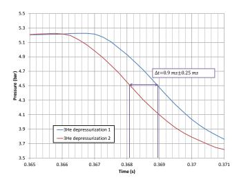
Fig. 4. Difference between 2 VABT01 opening times on 2 commissioning tests in the same conditions
