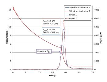
Fig. 5. Comparison of the two power transients resulting from the 2 similar depressurizations
