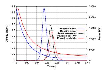
Fig. 6. Effect of density model on the power transient calculation
