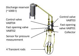
Fig. 2. Main components of the CABRI transient rods
