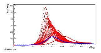
Fig. 14. Uncertainty propagation on the 1.3 bar case with the SPARTE code launched by URANIE  $% \left( {{{\rm{SPARTE}}} \right)$
