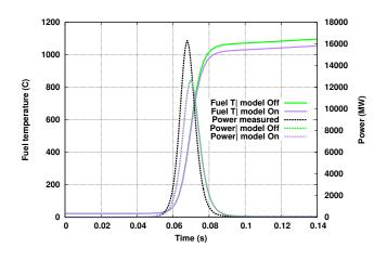
Fig. 10. Effect of axial distribution on the power transient calculation
