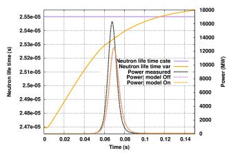
Fig. 11. Effect of neutron lifetime variability on the power transient calculation
