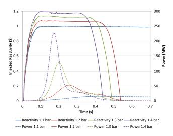
Fig. 13. Effect of small initial pressure variations on measured power transients
