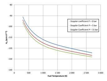
Fig. 7. Variability of the integral Doppler coefficient in CABRI core depending on fuel temperature and <sup>3</sup>He density
