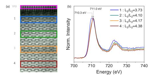
FIG. 8. (a) HAADF HR STEM image of the 32-nm GFO film highlighting four zones at various depths in the films, and (b) the Fe  $L_{2,3}$  EELS profiles integrated on these zones.
