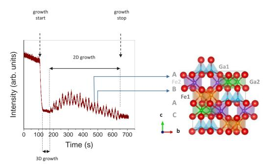
FIG. 2. Fluctuation of the intensity of a spot in the zero-order Laue zone during RHEED monitoring of the 7- nm GFO film growth. Each oscillation corresponds to the deposition of one fourth of a GFO cell, that is, to a layer of transition-metal/oxygen polyhedra.
