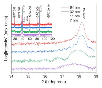
FIG. 3. X-ray diffractograms of the deposited GFO thin films in the  $\theta$ -2 $\theta$  mode, with a focus on the GFO 004 peak, the vertical line at  $2\theta = 38.17^{\circ}$  indicates the angle observed for bulk GFO x = 1.4 (c = 0.9422 nm) [17].
