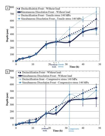
**Figure 9.** Influence of (a) tensile and (b) compressive mechanical loading on the depth of the dissolution of the  $\alpha$ , $\beta'$  brass CuZn40Pb2. In each graph, the effect of the mechanical loading is studied in comparison with the results obtained for the reference conditions (0.5 M NaNO<sub>3</sub>, pH 11, applied potential equal to 0.05 V/SCE without mechanical loading).
