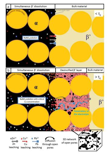
**Figure 10.** Schematic of the proposed dezincification mechanism (a) before  $t_c$  (b) after  $t_c$ .
