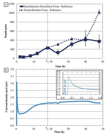
**Figure 4.** (a) dissolution depths (b) current density versus time curve during the dissolution tests of the  $\alpha,\beta'$  brass CuZn40Pb2 for the reference conditions (0.5 M NaNO<sub>3</sub> solution, with a pH adjusted to 11, and an applied potential equal to 0.05 V/SCE; without mechanical loading).
