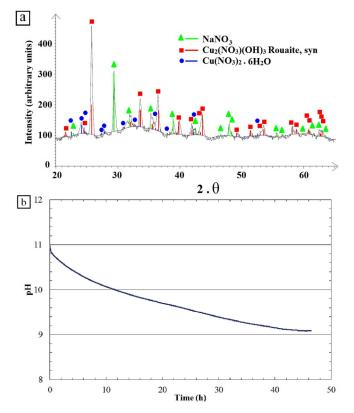
**Figure 5.** (a) XRD analysis of the blue corrosion products (b) pH vs. time during a dissolution test at the reference conditions, i.e., at 0.05 V/SCE in a 0.5 M NaNO<sub>3</sub> solution at pH 11, without mechanical loading, performed on  $\alpha$ , $\beta'$  brass CuZn40Pb2.
