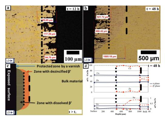
Figure 3. Analysis by optical microscope of a section of the  $\alpha,\beta'$ -brass CuZn40Pb2 sample after (a) a 12 h and (b) a 48 h dissolution test in a 0.5 M NaNO<sub>3</sub> solution at pH 11 under anodic polarization at 0.05 V/SCE. (c) Schematic of the corrosion damage and (d) EDX analysis.
