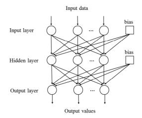
Figure 4 Layout of a three-layered, feed-forward Artificial Neural Network.
