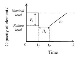
Figure 1 Evolution in time of the capacity of element *i*.
