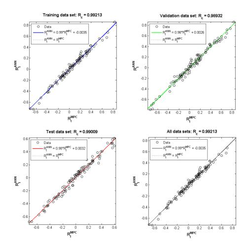
Figure 6. Linear regression between the network outputs (total resilience computed by the ANN model,  $R_t^{ANN}$ , on the vertical axis) and the original dynamic model outputs (total resilience,  $R_t^{MPC}$ , computed by the Model Predictive Control (MPC), on the horizontal axis).
