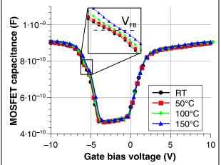
Fig. 3-4H-SiC planar MOSFET capacitance for different temperatures.
