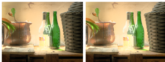
Fig. 3. GHE (left image); BBHE (right image) using "Bottles" HDR image.
