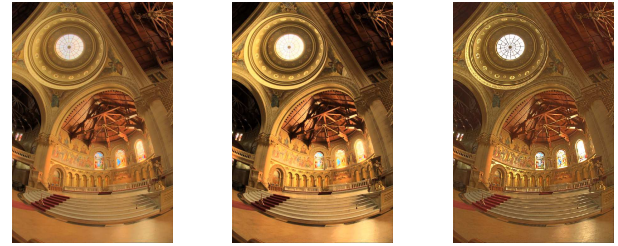
Fig. 3: "Memorial" HDR test image (18.38 f-stops) - Left image: proposed (5 levels, TMQI=0.951); Middle image: "Duan" (TMQI=0.935); Right image: "Fattal" (TMQI=0.927).
