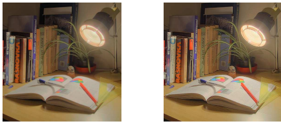
Fig. 2: "Light" HDR test image (17.46 f-stops) - Left image: proposed optimized \beta (1 level Norm 1, TMQI=0.920); Right image: proposed \beta = 0.25 (TMQI=0.813).
