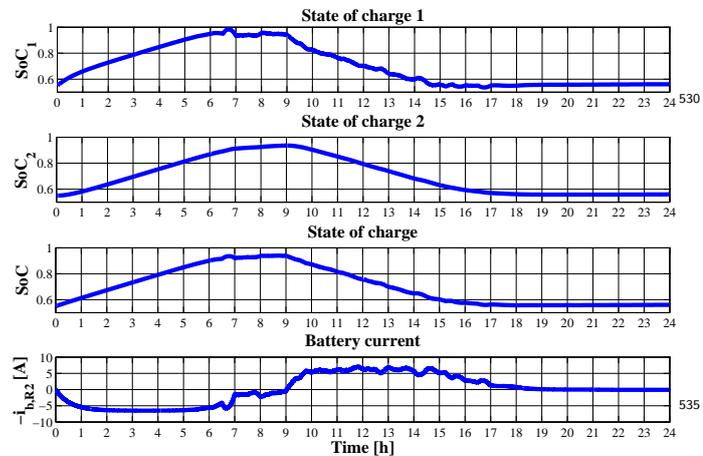
Figure 12: Scenario 1: battery state of charges ( $SoC_1, SoC_2, SoC$  as defined in (35)) and discharge current (perturbation scenario).
