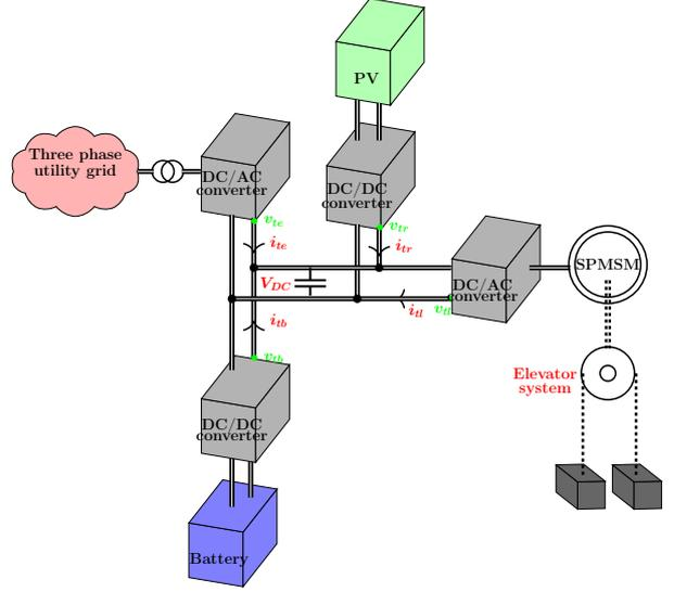
Figure 1: DC microgrid elevator system.
