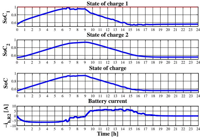
Figure 9: Nominal scenario: battery state of charges ( $SoC_1$ ,  $SoC_2$ ,  $SoC$  as defined in (35)) and discharge current.
