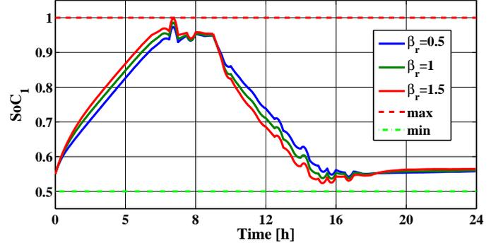
Figure 16: Scenario 5:  $SoC_1$  of the battery, as defined in (35a), with proportional uncertainties of the resistors as in (41).
