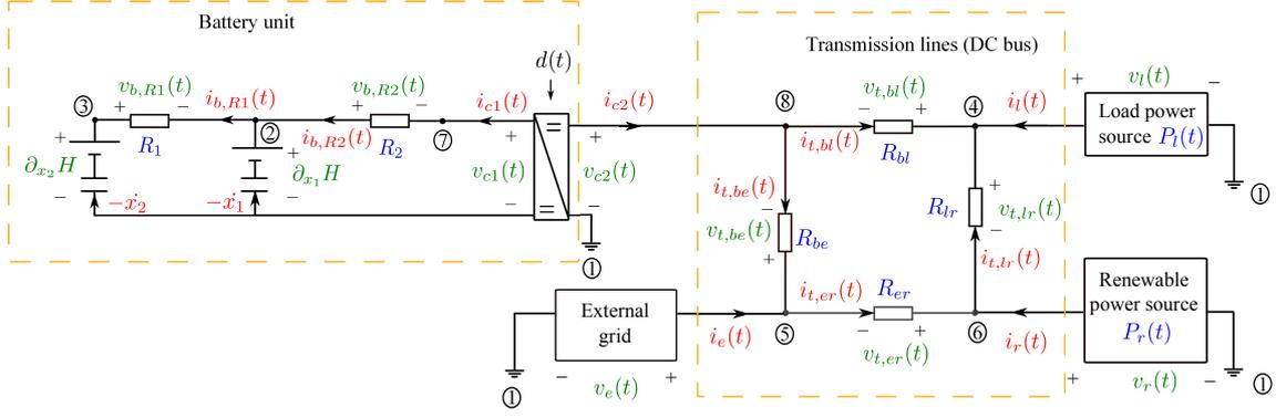
Figure 2: Electrical circuit of the DC microgrid.
