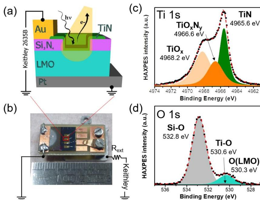
**Figure 1** (a) sample description (b) picture of a mounted sample (c)(d)HAXPES spectra of Ti 1s and O 1s for the stack  $\text{TiO}_x/\text{TiN}/\text{TiO}_x\text{N}_y/\text{LaMnO}_{3+\delta}$  in the initial resistance state at 0V.
