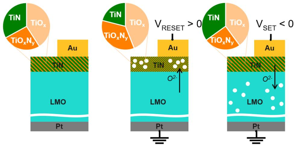
**Figure 3.** Sketch of the proposed oxygen exchange process occurring during RESET ( $V_{SET} > 0$ ) and SET ( $V_{RESET} < 0$ ). Inserts: the nominal composition of the TiN electrode based on the quantification of the Ti 1s area ratios shown in Figure3(c).
