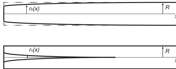
Figure 1. The negative bore concept: a negative plug is inserted in a cylindrical bore in order to provide the same open passage as that in a tapered bore. up : the geometry of a standard headjoint; down : a negative equivalent headjoint with the inserted plug.
