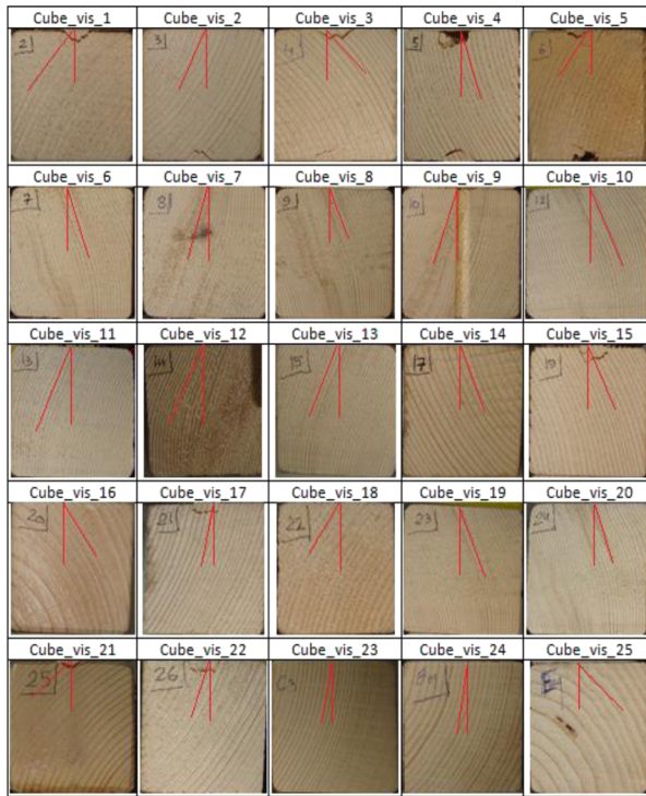
Fig. 9. 25 pictures of cube section – influence of the radial and ring orientation on the elastic behavior.
