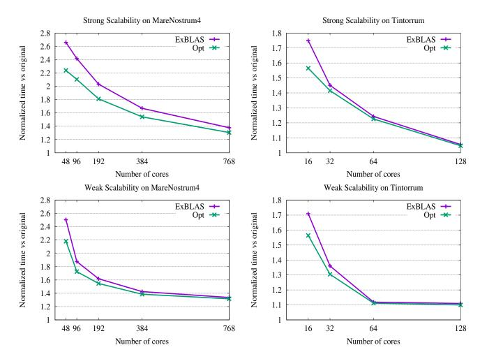
**Figure 4.** Analysis of the strong (top) and weak (bottom) scalability of the two reproducible versions of the MPI + OpenMP tasks PCG; the time is normalized with respect to the regular non-deterministic MPI version.
