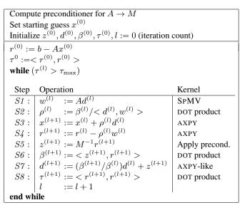
**Figure 1.** Formulation of the PCG solver annotated with computational kernels. The threshold  $\tau_{\rm max}$  is an upper bound on the relative residual for the computed approximation to the solution. In the notation,  $<\cdot,\cdot>$  computes the DOT (inner) product of its vector arguments.
