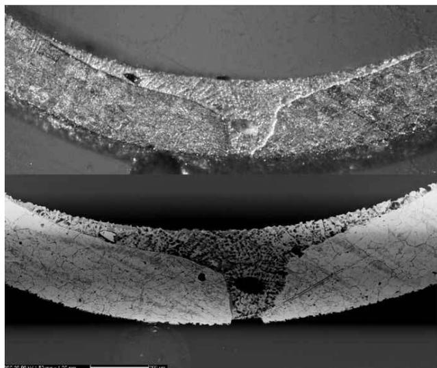
Figure 4: (See colour plate) (a) Optical and (b) SEM-BSE images of polished and aqua regia etched area of joint in ring. Scale bar is 200 microns.
