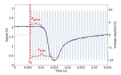
Fig. 5. Transmitted signal along the extraordinary axis from a L=9 $\mu$ m cell at  $V_0 = 0V$  (blue line). Grey line represents the electric field applied.  $\tau_{min}$  and  $\tau_{prec}$  are indicated.
