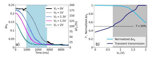
Fig. 8. a)  $\Delta n_g$  and  $\Delta \tau_g$  plotted as a function of acquisition time for different  $V_0$  (0V, 1V, 1.3V, 1.5V); the blue area is associated to the  $V_0=0$  measurement and indicates that for this voltage step the Fourier Transform is not possible in this time interval. b) Comparison between  $\Delta n_g$  normalized and the transient transmission T as a function of  $V_0$  (the curve is extrapolated from the experimental data). In gray the condition of T=50%
