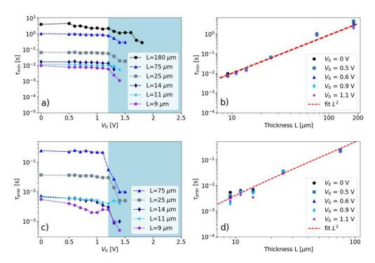
Fig. 6. Temporal dynamical features of the Fréedericksz transition.  $\tau_{min}$  evolution as a function of  $V_0$  and thickness (a, b),  $\tau_{prec}$  as a function of  $V_0$  and thickness (c, d). The area beyond the  $V_{th}$  (1.2V) is highlighted in blue (a,c) and the red line (b,d) indicates a quadratic fit of the data.
