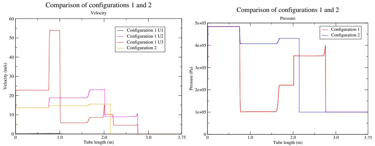
Figure 20: Comparison of Configurations 1 and 2 - Velocity (left) and pressure (right) profiles at  $t = 1.2$  ms
