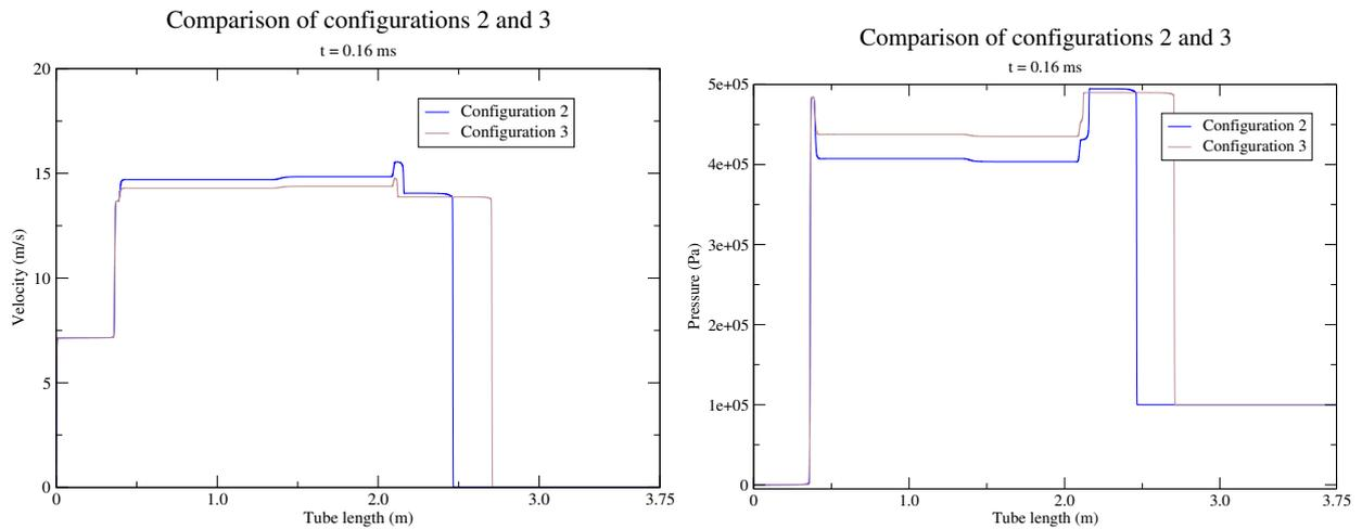
Figure 21: Comparison of Configurations 2 and 3 - Velocity (left) and pressure (right) profiles at  $t = 1.6$  ms
