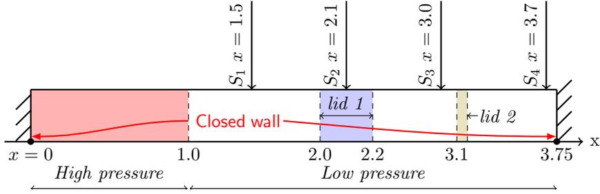
Figure 18: Scheme of the three-phase shock tube
