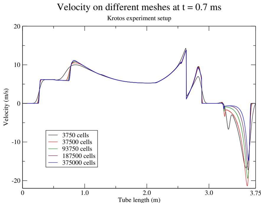
Figure 15: *Velocity at t = 0.7 ms on various meshes*
