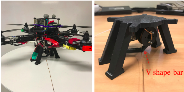
Fig. 9. The quadrotor body with Fig. 10. Winch prototype and sup-embedded winch for experiments port
