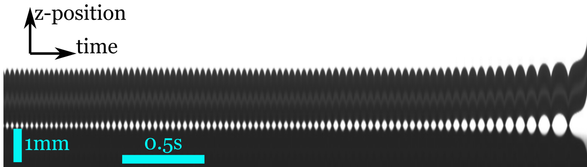
Fig. 3 Space-time diagram along the z axis passing through the center of the droplet and its mirror image on the silicon wafer (movie in the supplementary material†). The last 3.5 seconds are displayed and illustrate the multiple bounces that occur before the final take-off. In this experiment d = 6.1 mm.
