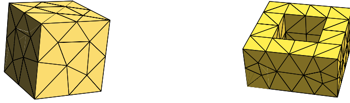
Figure 1: The two model geometries rendered with the coarsest triangular surface meshes used in the computations
