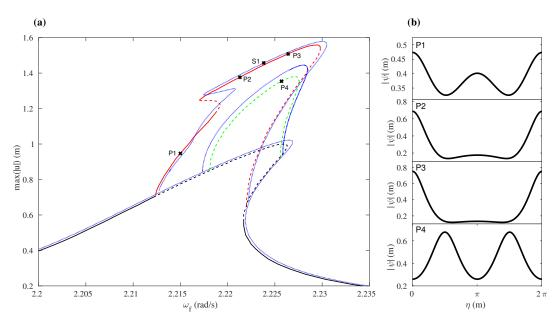
Figure 1: Panel (a) shows the bifurcation diagram computed with the NLSE and the HBM approaches. For the NLSE, solid lines show stable solutions while dashed lines identify unstable ones. Blue dotted lines show results obtained from the HBM approach. Panel (b) shows the envelope functions calculated with the NLSE.
