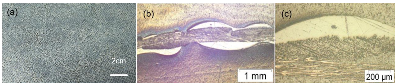
Fig. 1. Powdered carbon/PEEK fabric. (a) Macroscopic view; (b) and (c) cross-section microstructure of the powdered fabric.
